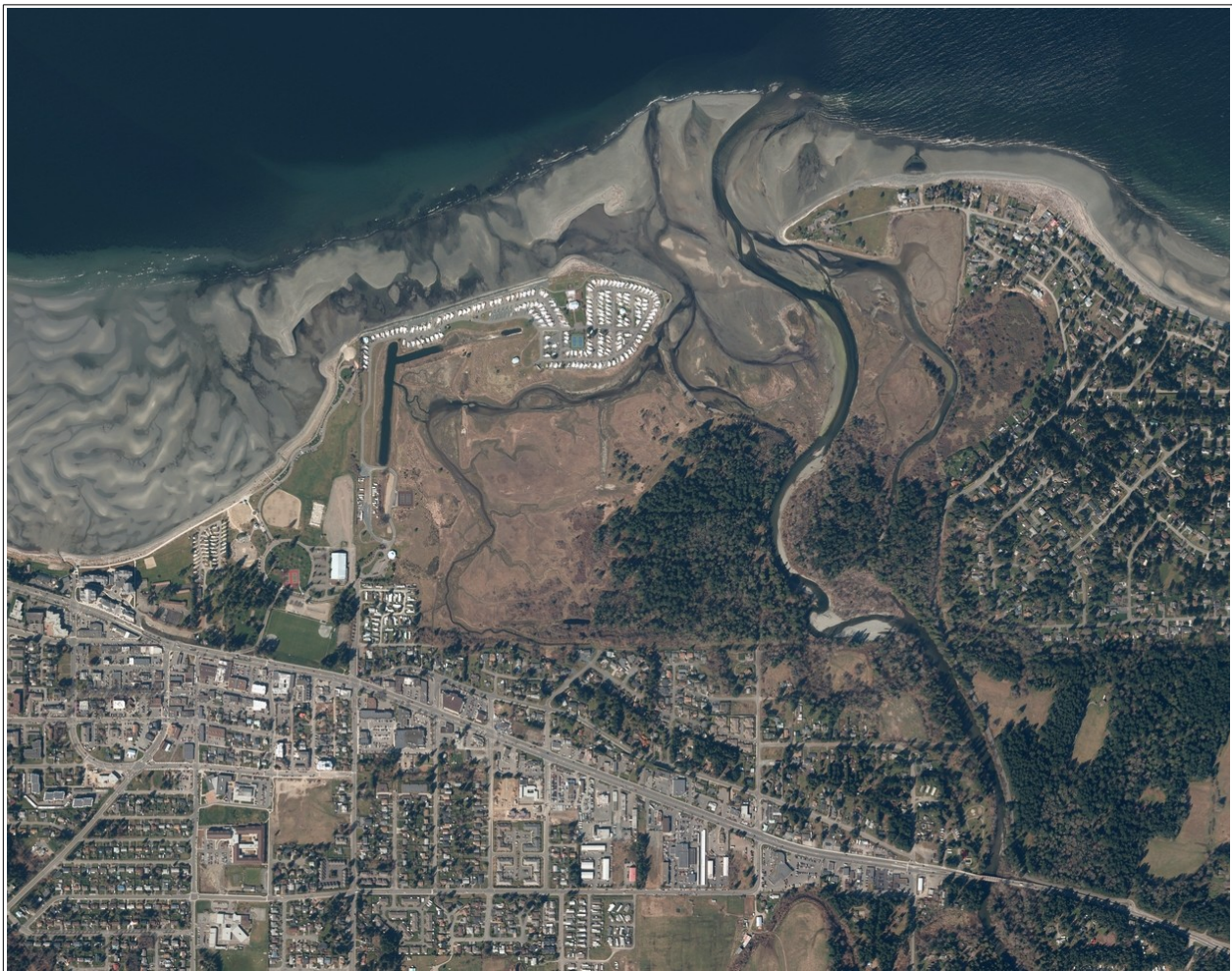
Figure 20. Typical Salish sediments found in the modern delta of the Englishman River at Parksville. The river is largely re-transporting older glaciofluvial deposits which are then redistributed by wave action in sea, as seen in the intertidal zone. The image shows a 3 km width.
