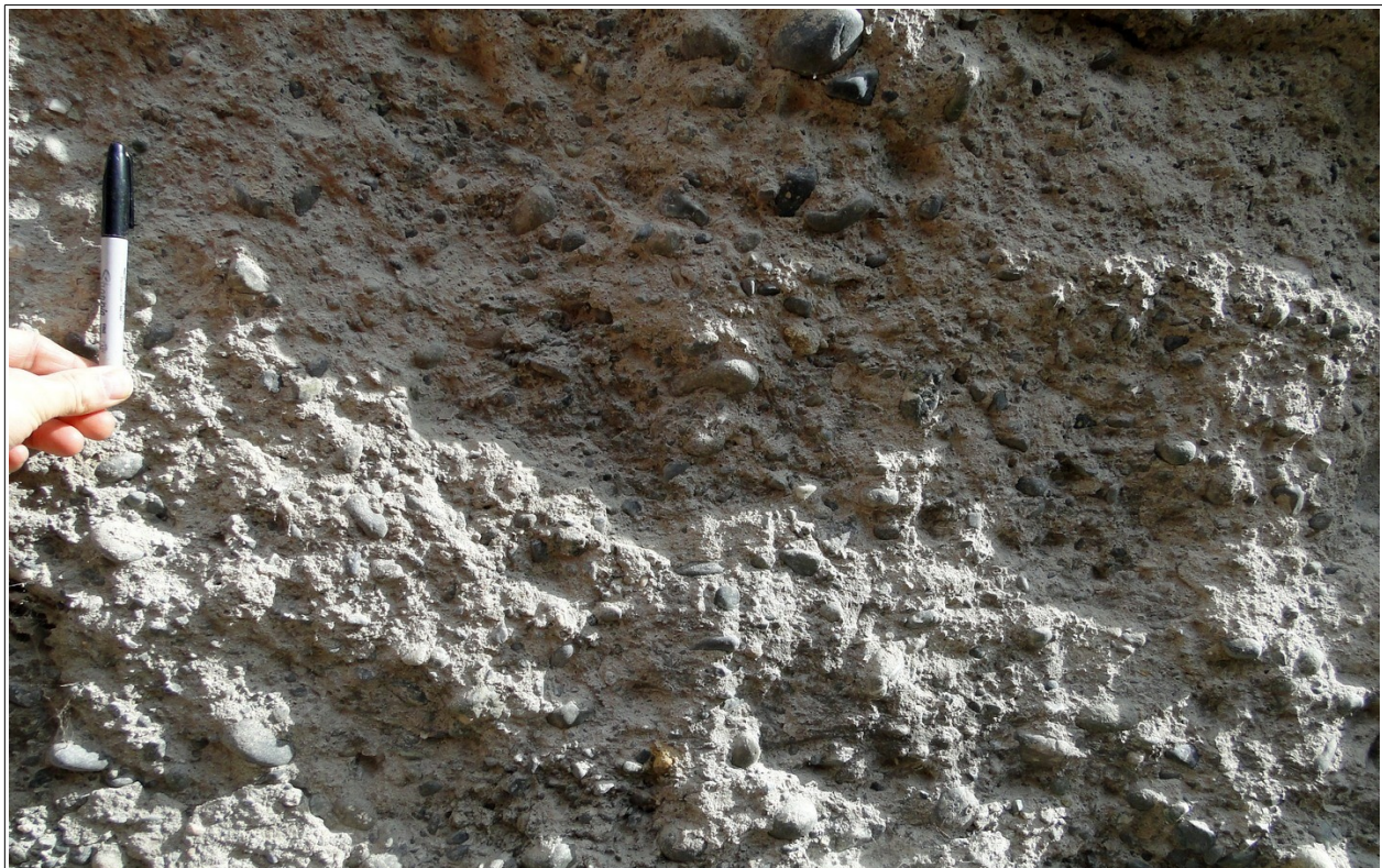
Figure 15. Gravelly facies of Vashon Drift. Interstratified diamicton and massive matrix supported gravel exposed along French Creek at the Qualicum Beach airport. The 5 m thick unit has a sandy matrix enclosing mainly well-rounded pebbles, cobbles and occasional boulders. The drift overlies at least 5 m of light brown Quadra Sand at the base of the section.
